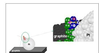
Figure 4. O-atom in SO<sub>3</sub><sup>-</sup> orientation and coordination with Pt nanoparticle [1]
