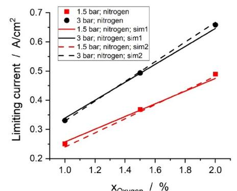
Figure 9. Validation with limiting current analysis
