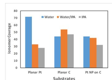
Figure 2. Effect of dispersion media on ionomer coverage on different substrates.
